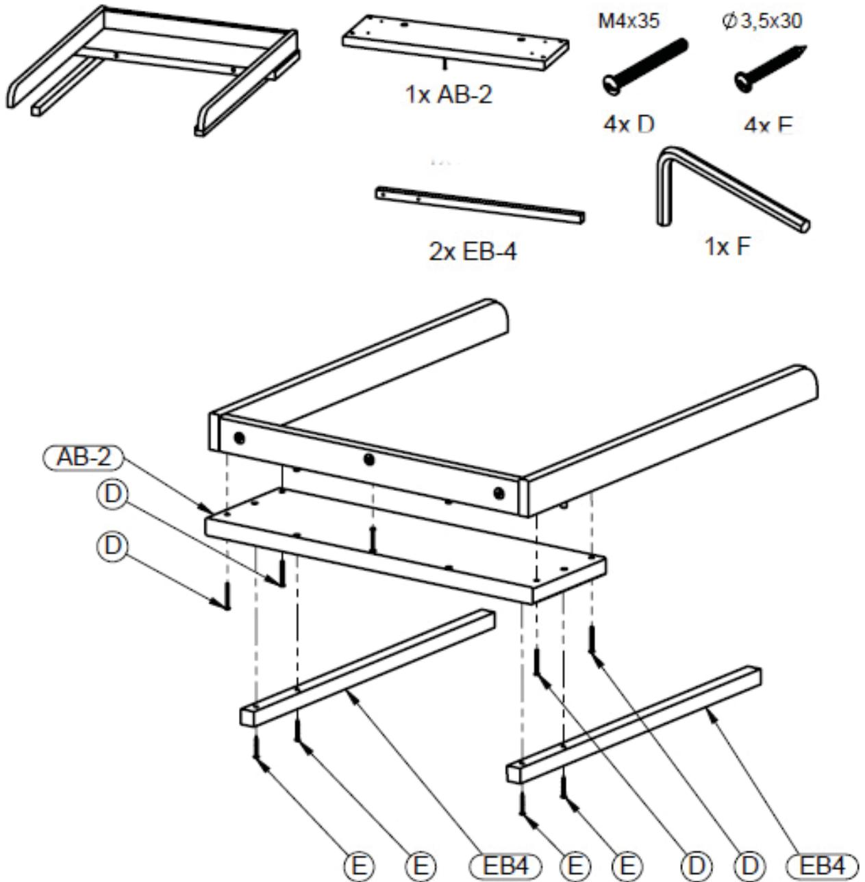
**Step 5 :** Use the parts of step 4, the base **AB2**, both supports **EP4**, four wood screws **D** and four wood screws **E**
