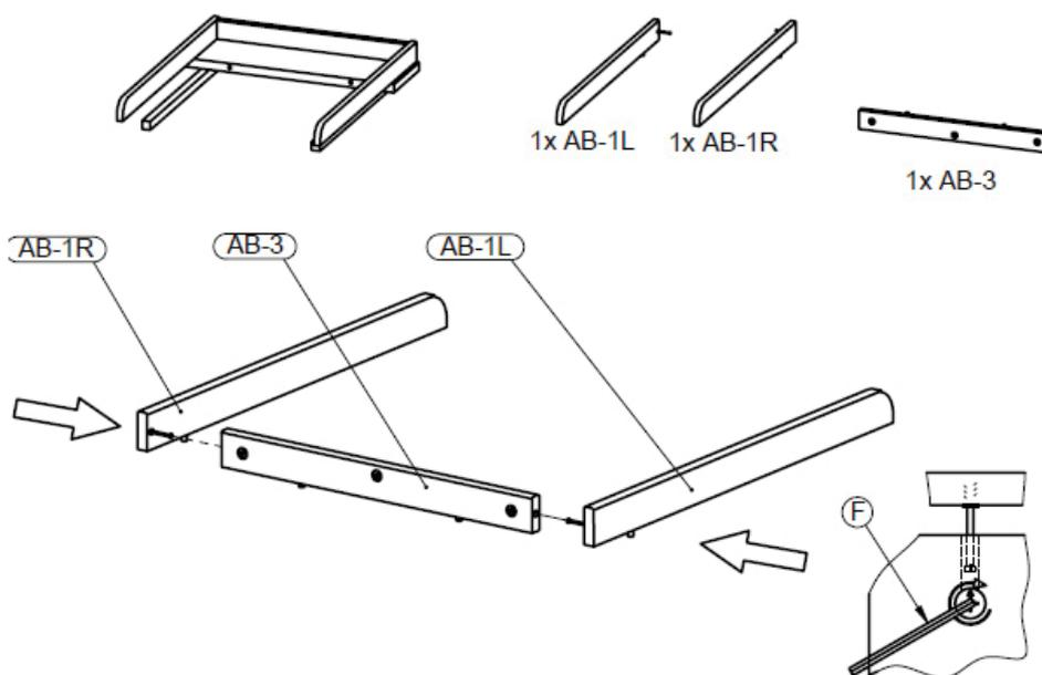
**Step 4 :** Use the assembled parts **AB1 (L and R)** and **AB3**
