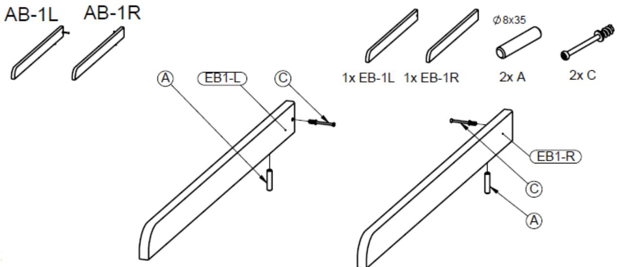
**Step 1 :** Use both sides **EB1 (L and R)**, two wooden dowels **A** and two connectors **C**
