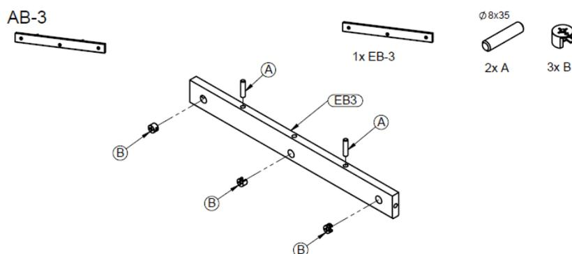
**Step 3 :** Use the back **EB3**, two wooden dowels **A** and three eccentrics **B**
