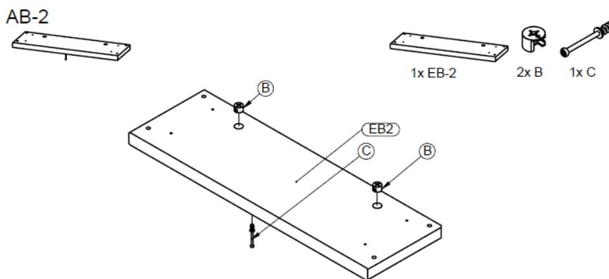
**Step 2 :** Use the base **EB2**, one connector **C** and two eccentrics **B**
